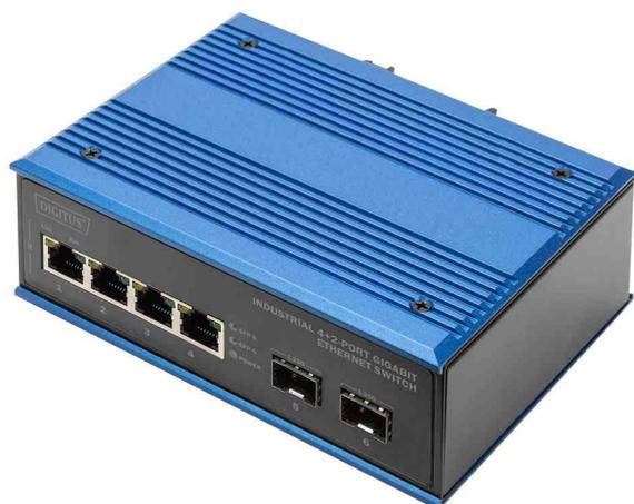
Industrial Gigabit Ethernet Switch, 4+2 Ports
